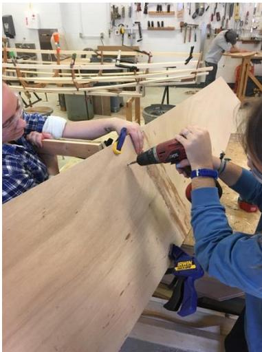
presented. We had two people holding the piece being attached, another holding the side plank in place, and one more predrilling holes and screwing everything together. After several failed attempts at different bracing practices, we were able to find the best position to place clamps. Having the clamps in place made it easier to align the frames and bulkheads to our marks.
